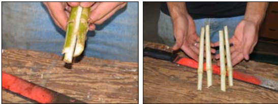
Quartering is a quick and easy way to ensure that a quality sample arrives at the laboratory.
